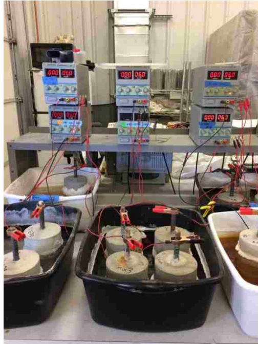
Figure 2. 8: Accelerated Corrosion Setup
